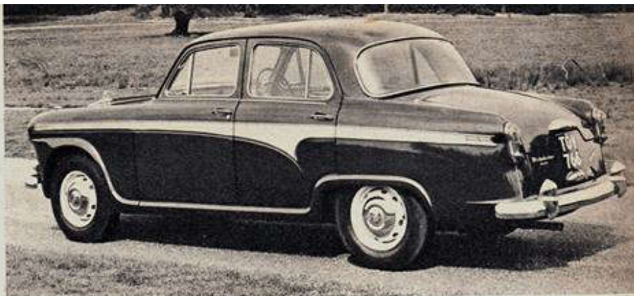
BROAD and curved, the rear window is big enough to make reversing easy. Direction signal flashers have amber lenses, spaced apart from the red stop and tail lamps.
